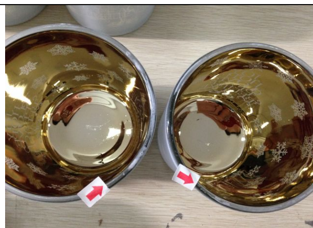
19 1047 defect white coating on the edge
